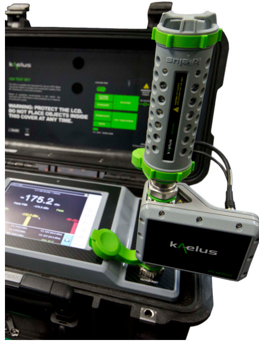
Figure 6 RTF module on the iQA (CIS-0001A PIM Source used for 5th order calibration)
