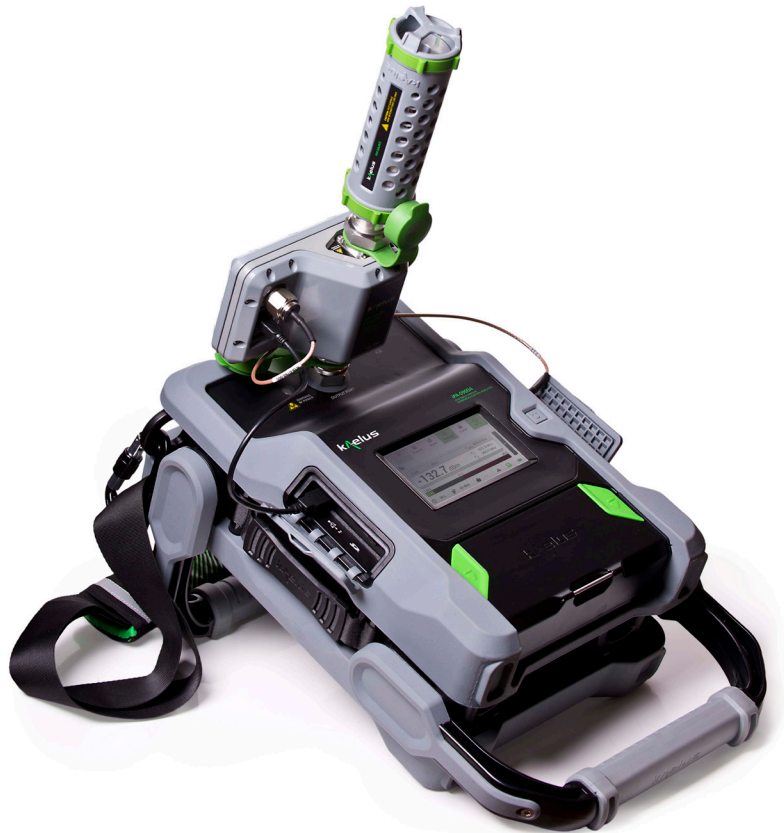
Figure 7 RTF module attached to iPA with PIM Source attached to Test port
