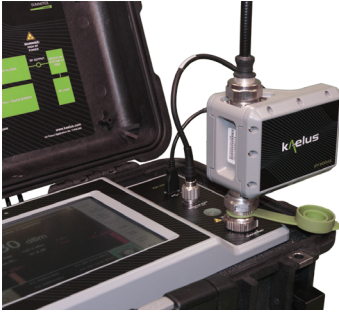
Range to Fault (RTF) Module
