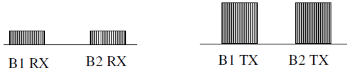
Figure 10 Typical Spectrum of Passive Type 3 Combiner (at both antenna ports)
