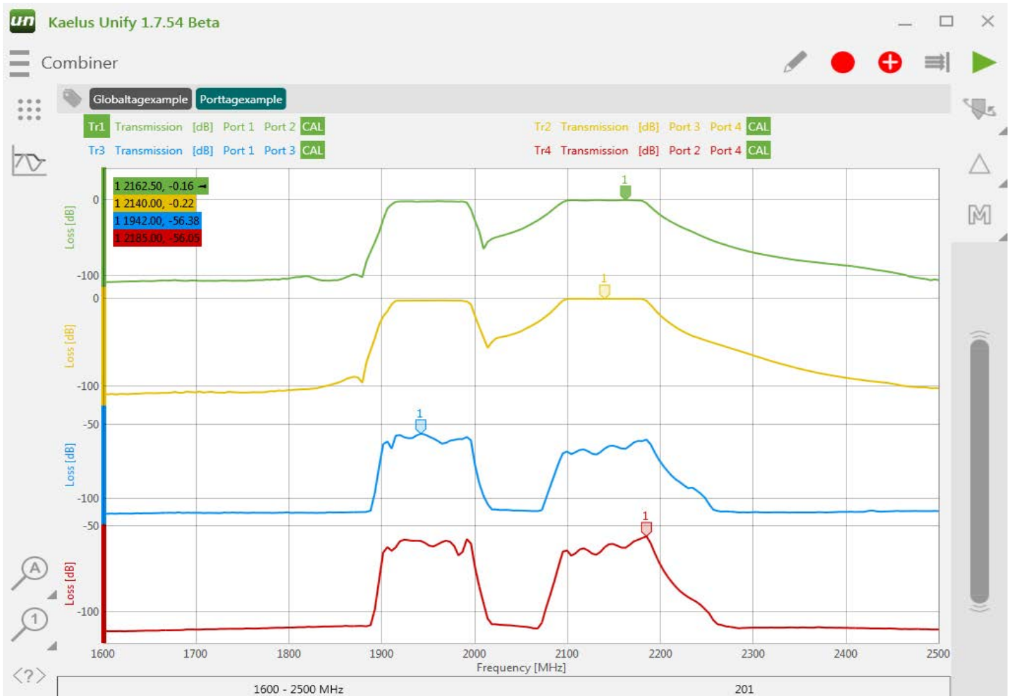
Figure 33 Four Port Analysis Using 4 iVA's and Transmission Mode
