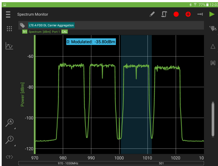
Figure 2. Measurement of RF power of third component carrier in an LTE-Advanced FDD downlink signal with 4 component carriers.
