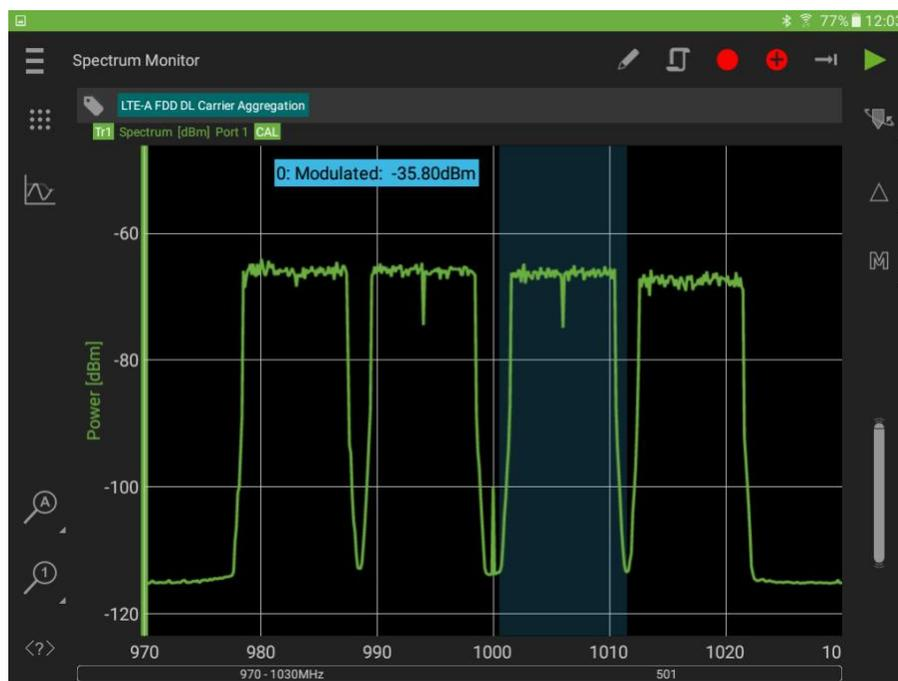
Figure 2. Measurement of RF power of third component carrier in an LTE-Advanced FDD downlink signal with 4 component carriers.
