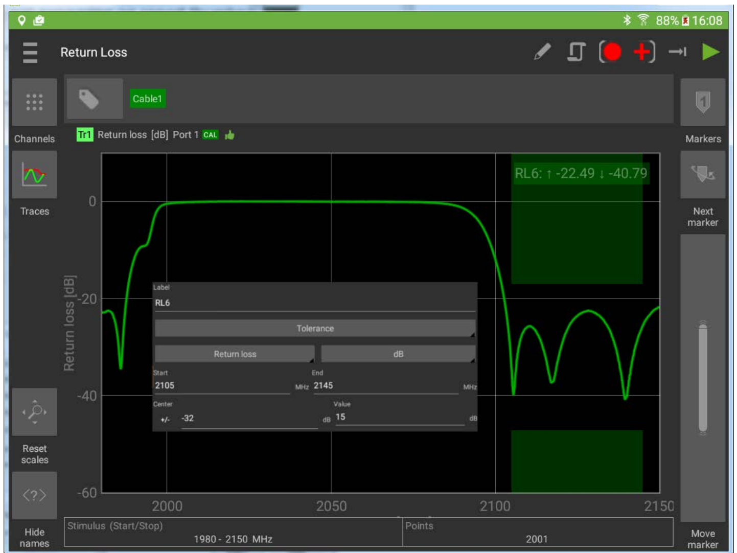
Figure 21 Tolerance Spec Limit
