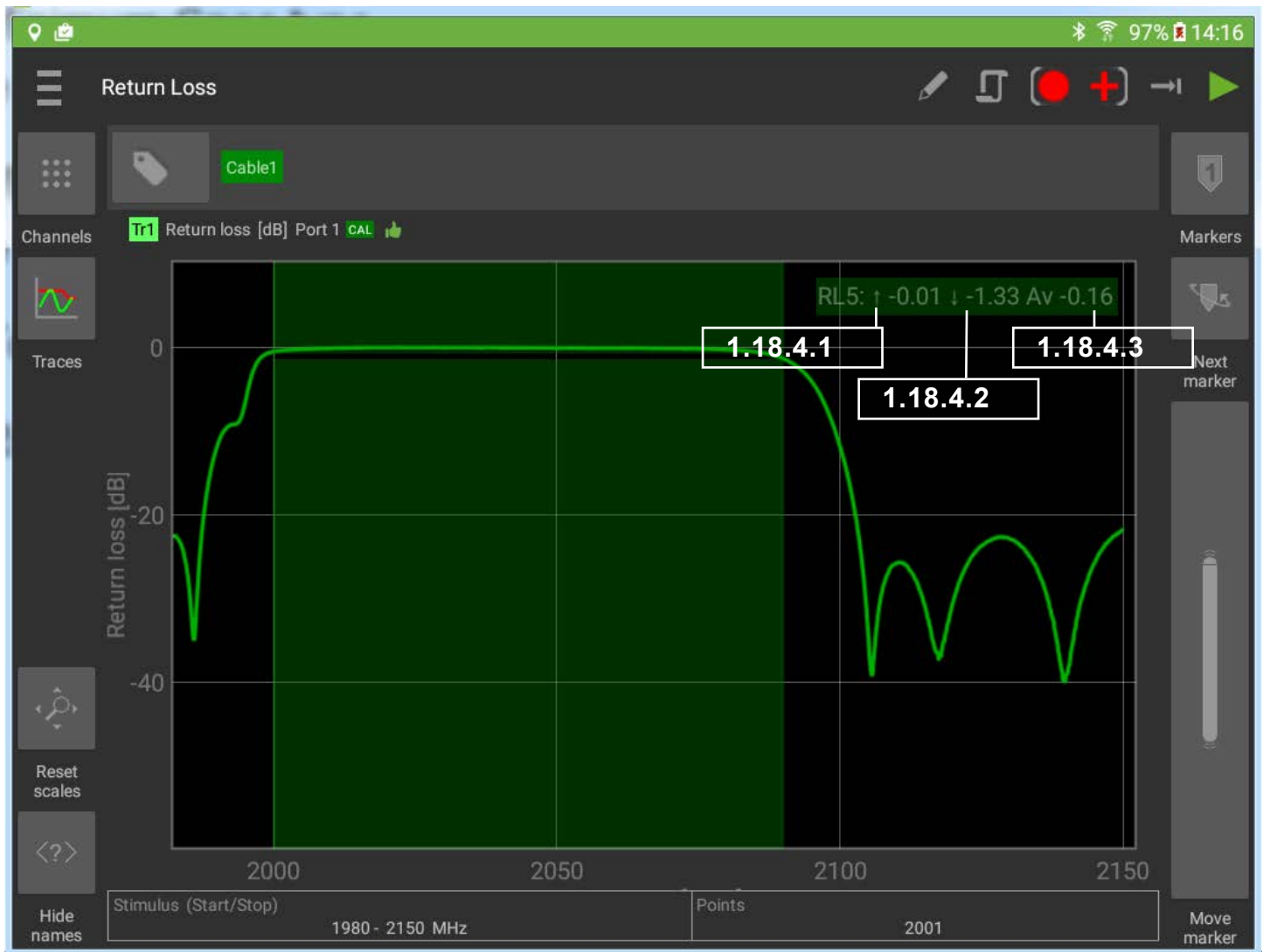
Figure 20 Ripple Limit on a Trace
