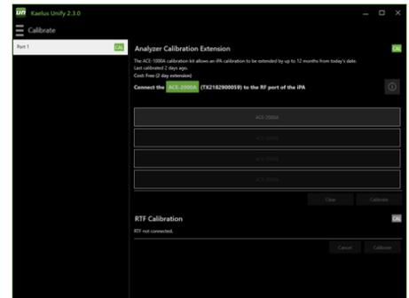
1. Ensure the iPA or iTA is connected via one of the connection options. Scan for the iPA or iTA in device call out if it is not already shown. Connect by clicking on the blue Wi-Fi symbol on the device. Click CAL.
