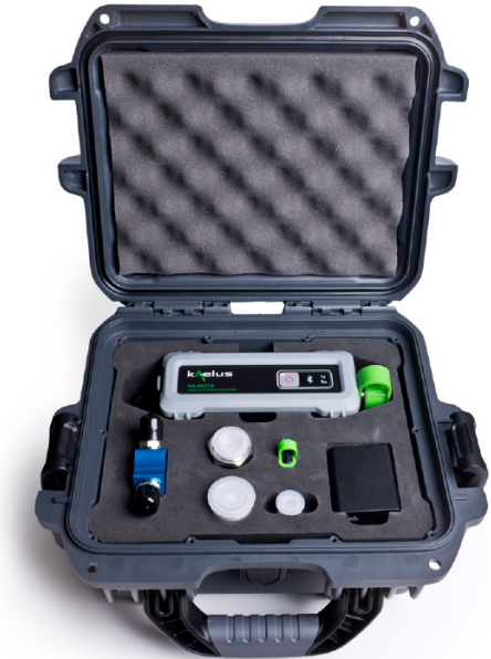
A single case can accommodate 1x iVA, 1x OSL and 1x adaptor kit
