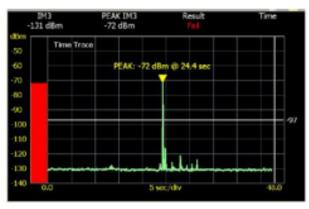
Dynamic testing identifies loose metal-to-metal connections as well as contact surface defects that might cause arcing at higher power levels. Without dynamic testing these
