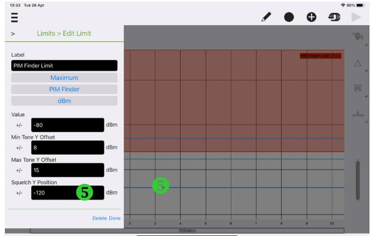
Now that the iVA is correctly set up, turn on the iPA transmitter and start sweeping the PIM probe on the arc distance measured by the RTF. Listen to the Theremin sound and mark the position(s) where the PIM centers were identified. Focussing on each of the PIM centers, orient the probe at different angles to confirm its location.
