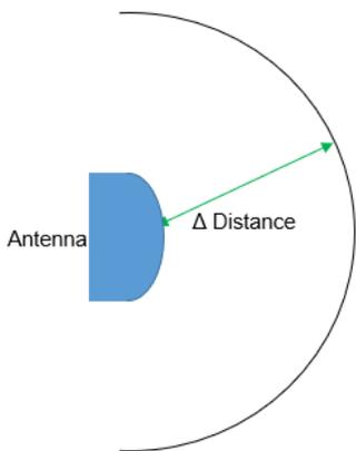
Using the RTF, we can extract the distance of the strongest PIM source in relation to the Antenna face, however, without the angle information, we can only assume it is located somewhere along the "Δ" distance arc from the antenna. We now need to identify the location of the PIM source using the PIM Finder probe.
