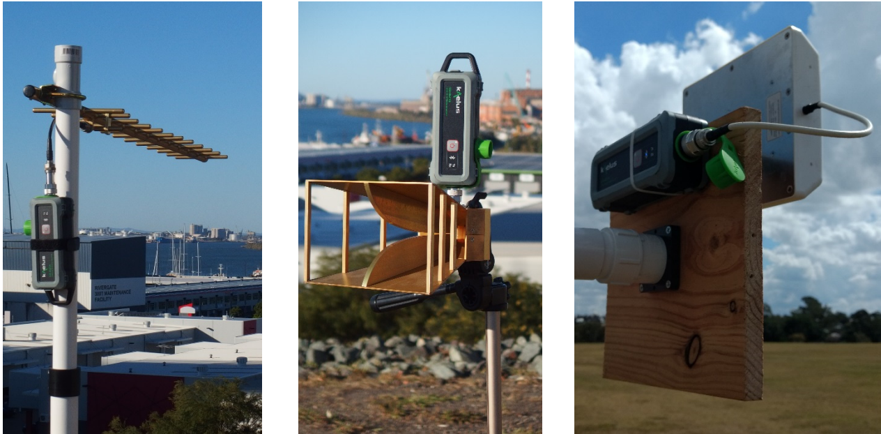
(a) iVA attached to antenna mast with velcro strap. (b) iVA connected directly to RF port of antenna. (c) iVA affixed to antenna mount with cable tie.
