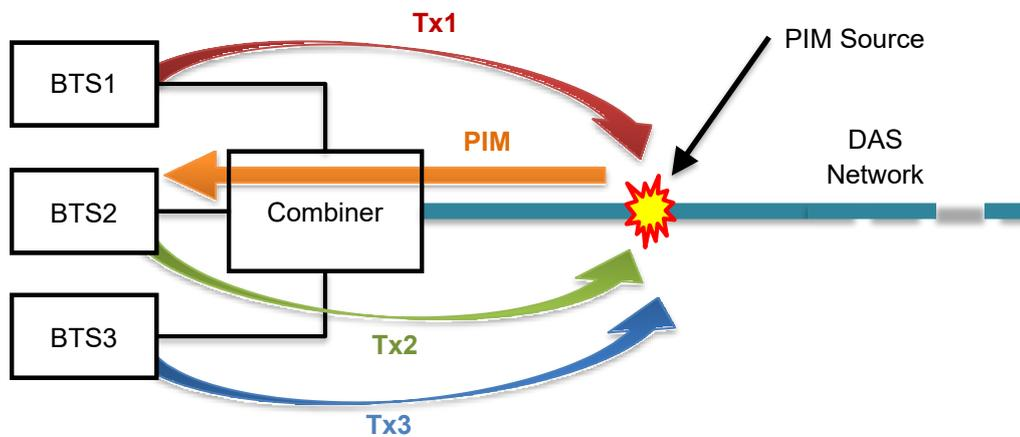
Figure 3. Illustration of cross-band PIM scenario in a passive DAS installation with three BTSs. Downlink carriers Tx1, Tx2 & Tx3 excite a PIM source in the common RF path, which then emits a PIM signal back towards the BTSs.
