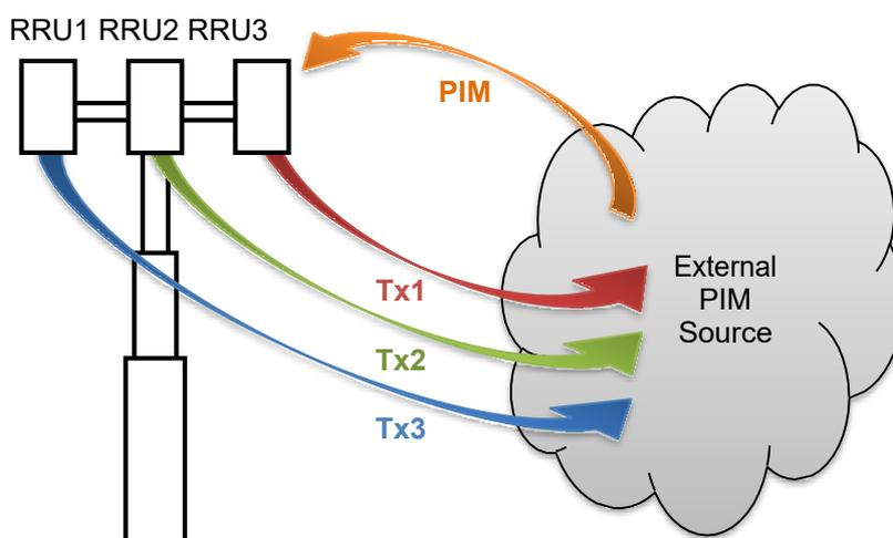
Figure 1. Illustration of cross-band PIM scenario involving 3 co-located RRU units. Downlink carriers Tx1, Tx2 & Tx3 illuminate an external PIM source, which then re-radiates PIM back towards the cell site.
