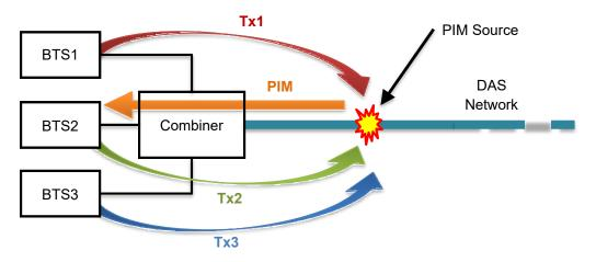
Figure 3. Illustration of cross-band PIM scenario in a passive DAS installation with three BTSs. Downlink carriers Tx1, Tx2 & Tx3 excite a PIM source in the common RF path, which then emits a PIM signal back towards the BTSs.
