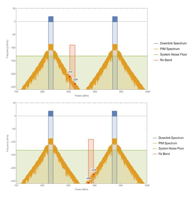
Figure 5: Signal Spectra for RRU1 and RRU2
