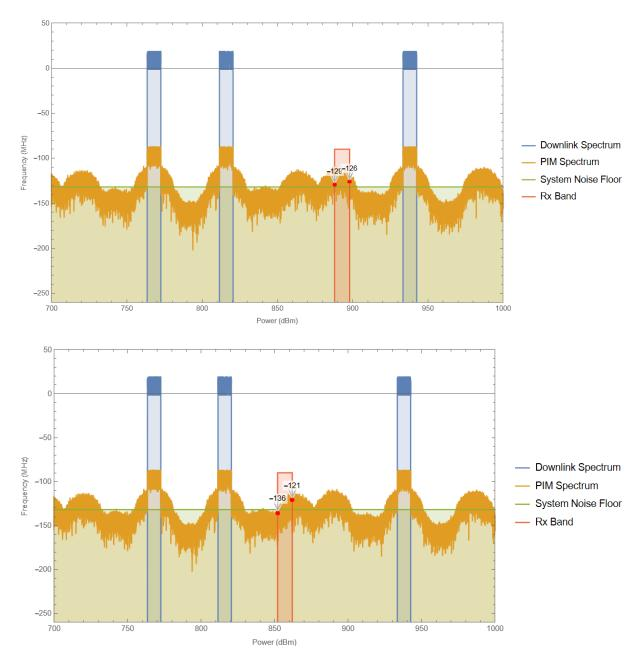
Figure 6: Signal Spectra when RRU3 is introduced
