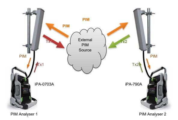
Figure 7. Typical equipment setup used to perform cross-band PIM testing on a cell site with two co-sited RRU systems.
