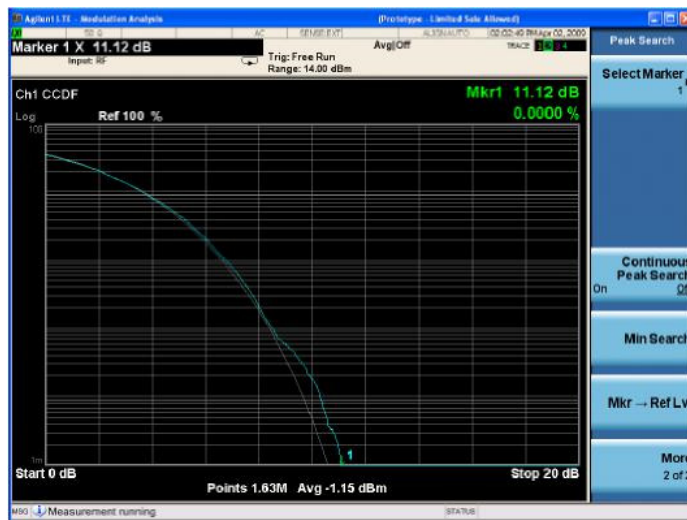
Figure 5 – CCDF of LTE downlink signal with 10 MHz bandwidth and 64QAM subcarrier modulation.
