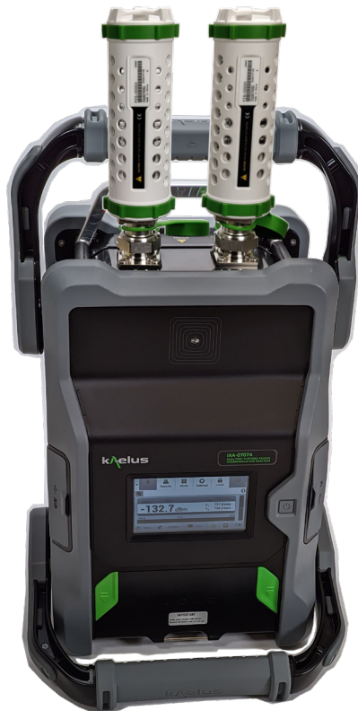
Figure 46 iXA With PIM Sources attached
