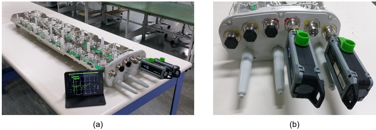
Figure 2. Equipment setup for an inter-band isolation test on a multiband sector antenna.
