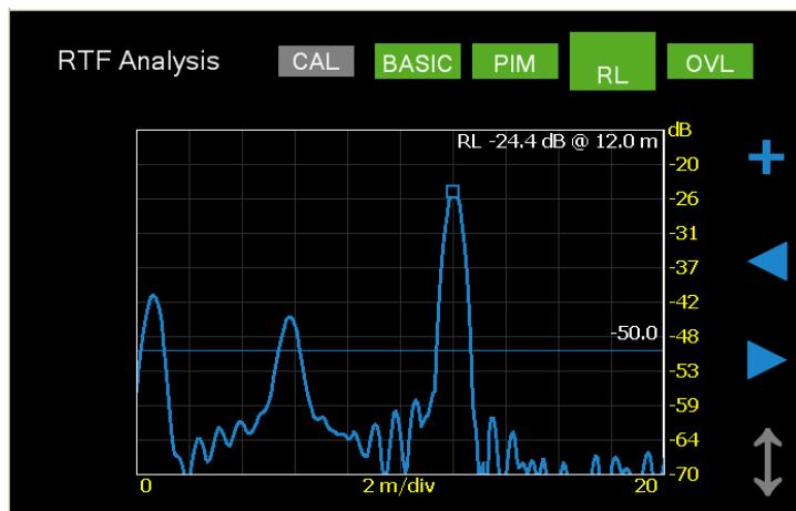
With a second button push, the operator can switch to “RL” view to see return loss vs. distance. As with the PIM view, a marker function is provided to display the magnitude and distance of each Return Loss peak.
